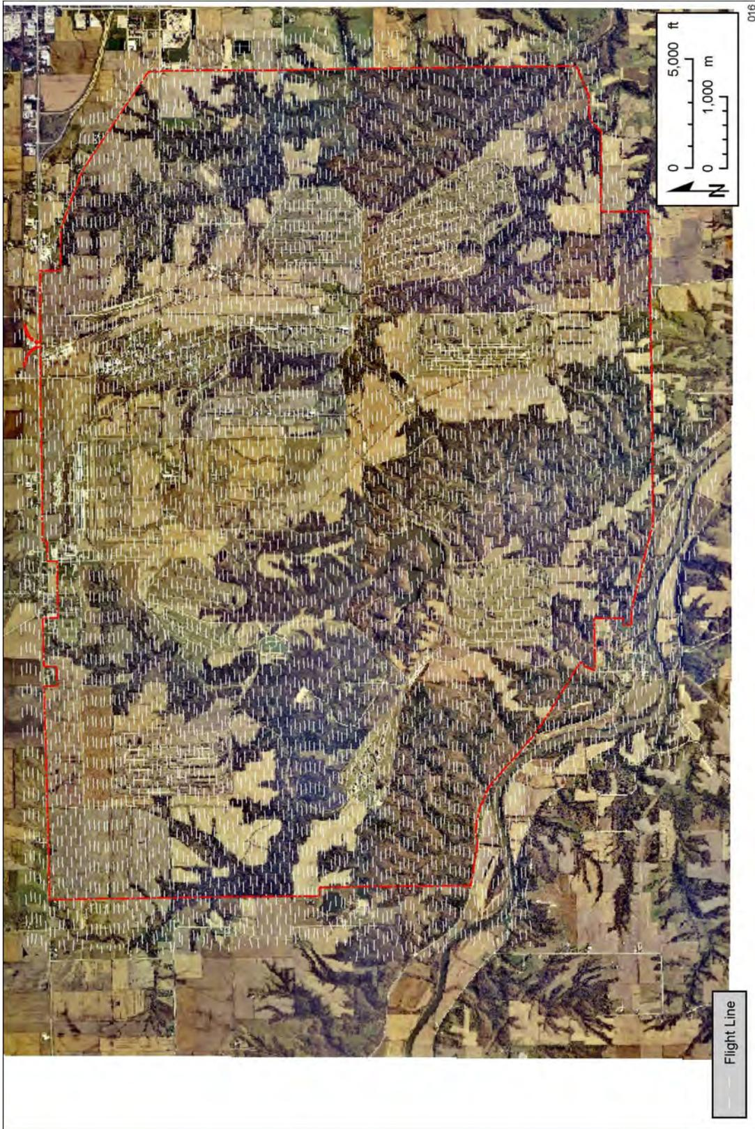
**Figure 5-1** Flight lines taken by the helicopter taken during the AMS aerial survey.
